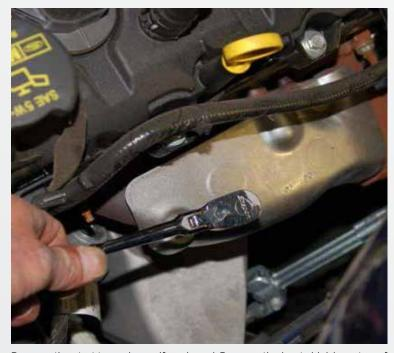
Remove the strut tower brace if equipped. Remove the heat shields on top of the stock exhaust manifolds. Unplug the front oxygen sensors at the back of the valve covers on each side of the engine.
