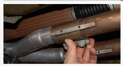
Install the provided studs into the collector flanges of the BBK Headers. Install the BBK X-Pipe kit.
