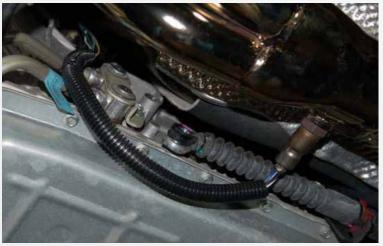
Remove the front oxygen sensors from the stock cat back pipe and install them into the BBK Full Length Header Collectors. Route the driver side oxygen sensor wires under the shift lever and zip tie to one of the steel Transmission cooler lines.
