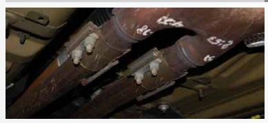
Loosen the 2 nuts on each of the barrel style clamps that connect the exhaust system to the stock X-Pipe. Remove the nuts at the exhaust manifold collectors and remove the entire X-Pipe assembly. From the top of the engine compartment, remove the stock nuts that bolt up the stock exhaust manifolds and remove from vehicle along with the stock gaskets.
